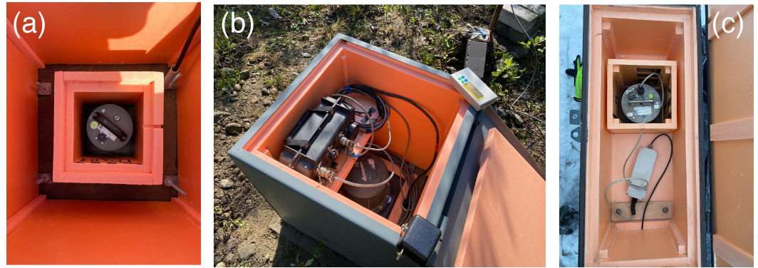
Figure 3. The seismic equipment within the insulated metal cases at stations Uмба (a), Verkhnetulomsky (b), and Ogni Murmanska (c).
