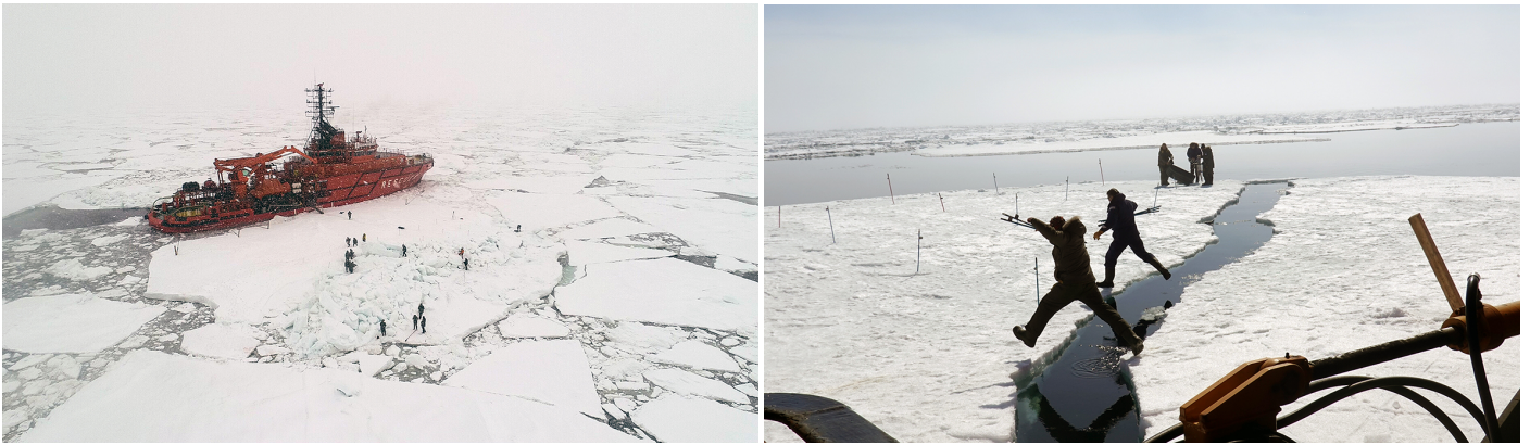
Figure 1. The most voluminous IF among the 22 investigated during the 2019 winter expedition was numbered 18 and was moored to an icebreaker on its starboard side. Length of the icebreaker is 73 meters and its beam athwartships is 15.5 meters. A photo was taken using a UAV (left). A crack on the IF numbered 14 formed due to swell arriving through drifting ice from the ice-free Pacific Ocean (right).
