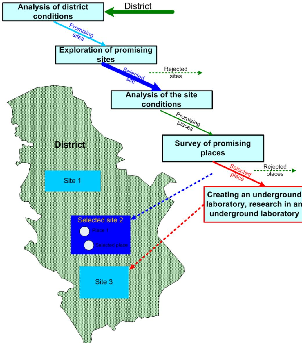
**Figure 1.** Stages of work to substantiate the suitability of the subsoil area for the radioactive waste repository facility [Gupalo et al., 2005].
