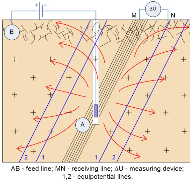
**Figure 5.** Functional diagram of the research using the charged body method.
