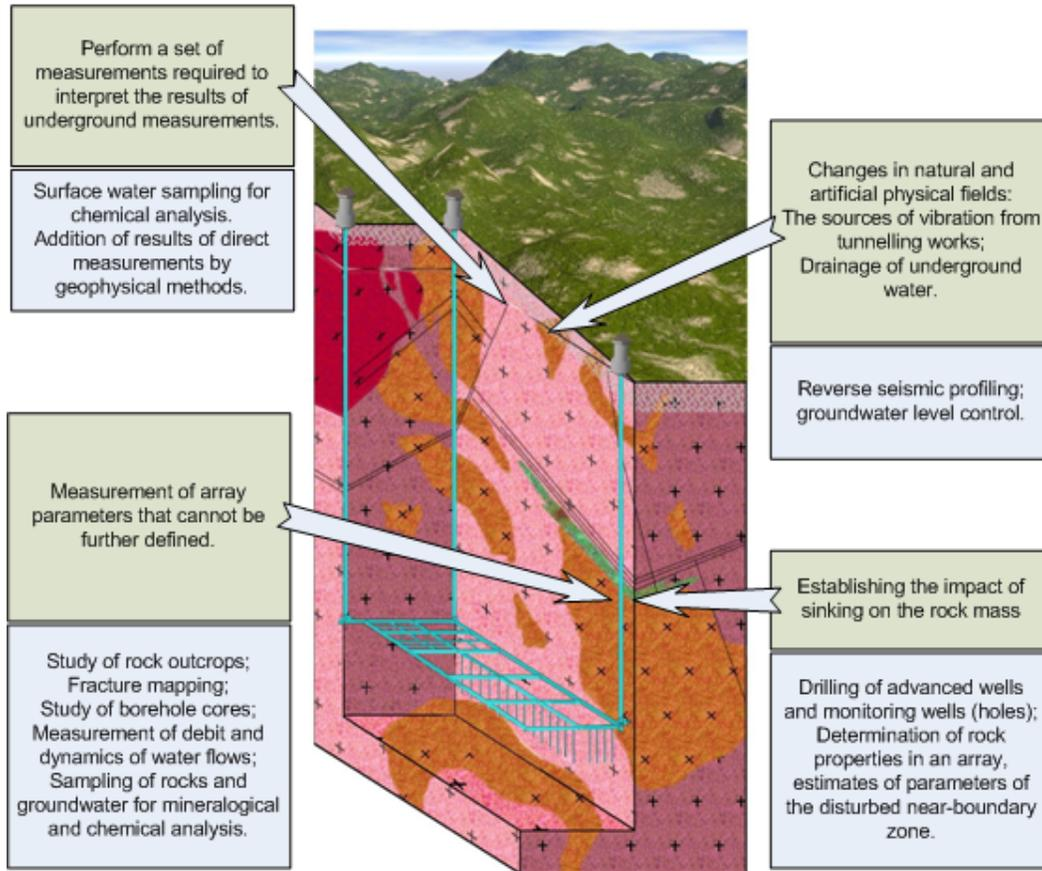
**Figure 6.** Combination of measuring and construction works.
