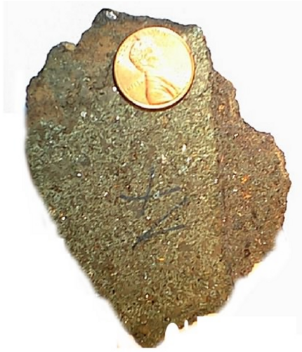
Figure 2. Sample of micaceous pyroxenite with clearly seen shiny mica flakes (49%) in a dark mass of clinopyroxene (50%). Scale: one penny coin.
