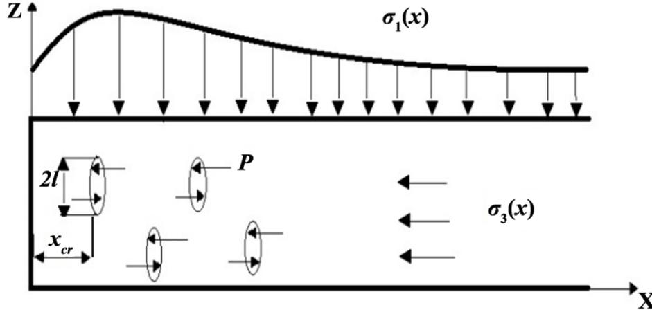
**Figure 2.** The coal seam ahead of the working face in the stress field  $\sigma_1(x) - \sigma_3(x)$ , weakened by the cracks filled with gas under pressure  $P$ .
