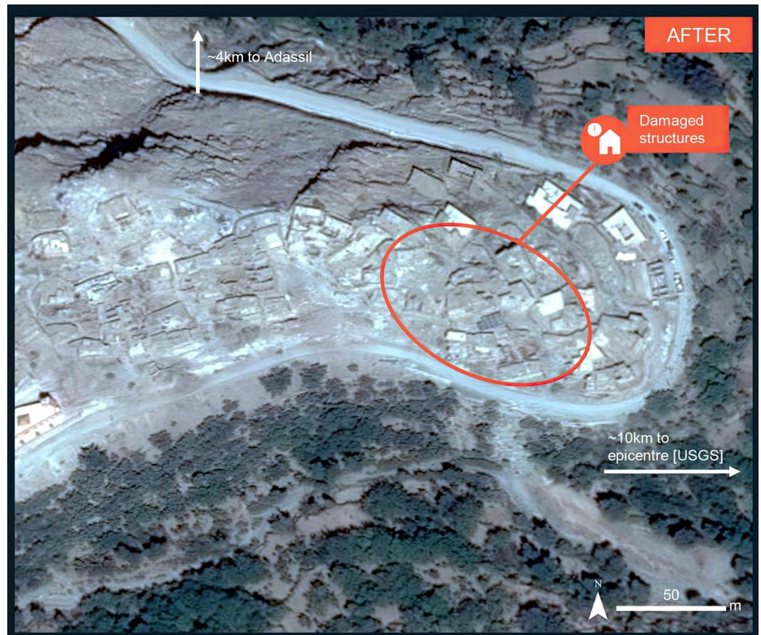
**Figure 12.** Observed damage in Targua. Source: United Nations Satellite Center, UNOSAT, Preliminary Assessment Report [UNOSAT, 2023].
