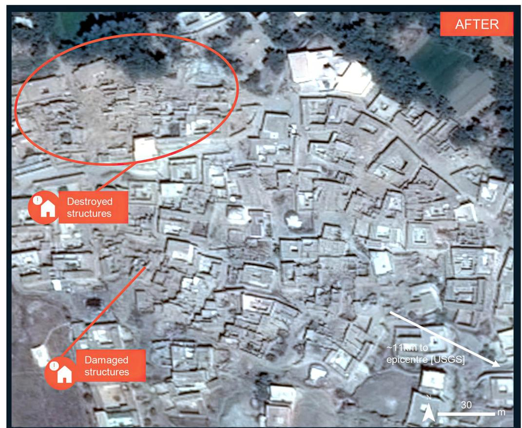
**Figure 11.** Observed damage in Adassil. Source: United Nations Satellite Center, UNOSAT, Preliminary Assessment Report [UNOSAT, 2023].
