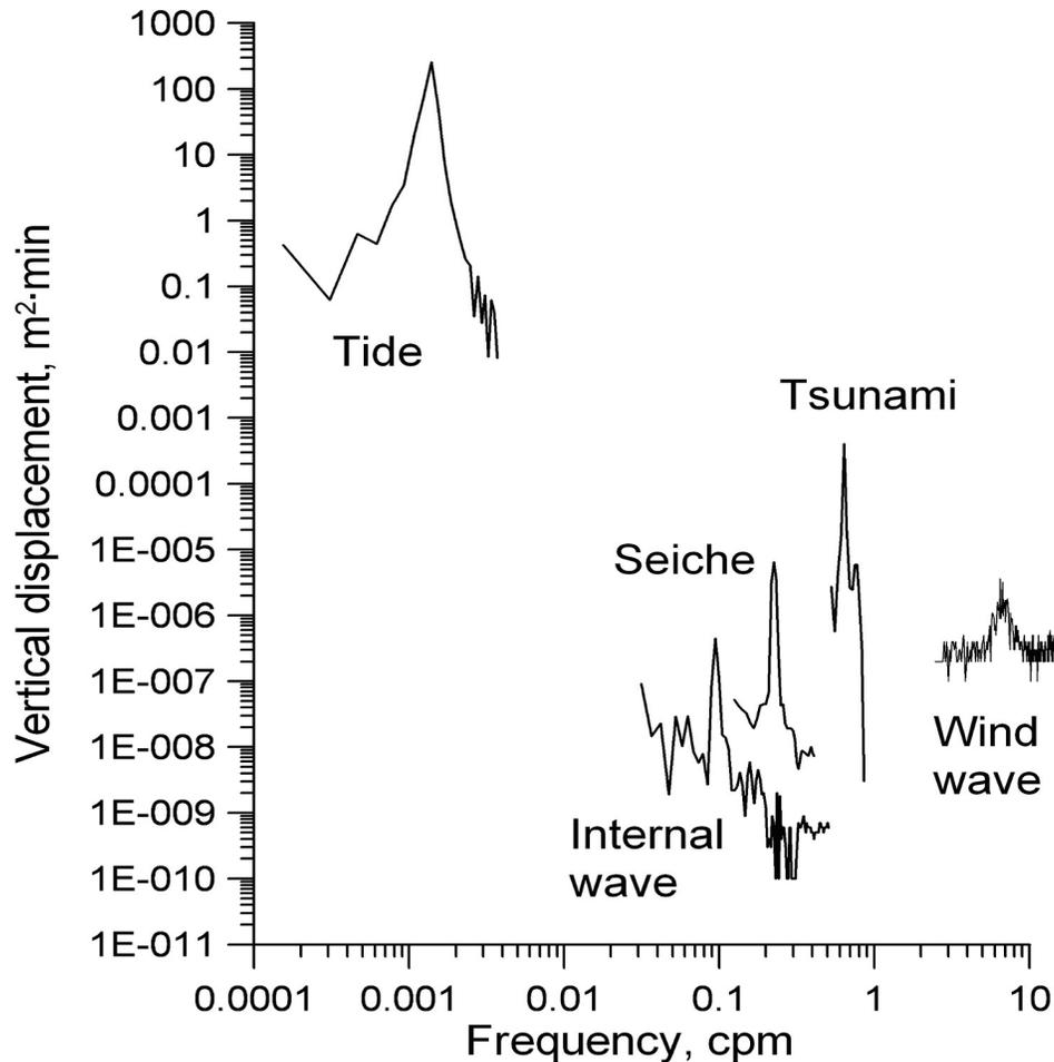
**Figure 1.** Combined spectra of the surface manifestation of five different wave processes measured under the ice cover in Spitsbergen fjords.
