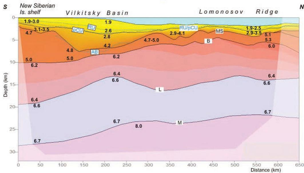
**Figure 6.** Velocity model of the Earth's crust along the Arctic-2007 profile [Poselov *et al.*, 2014]. RU is the Pre-Miocene regional unconformity, pCU is Post-Campanian unconformity, AB is acoustic basement, MS is the top of the metasedimentary layer, B is the top of the upper crust, L is the top of the lower crust, M is Moho, 6.1 are P-wave velocities (km/s), the dotted blue lines are main unconformities in the time-to-depth transformed seismic profile A-7.
