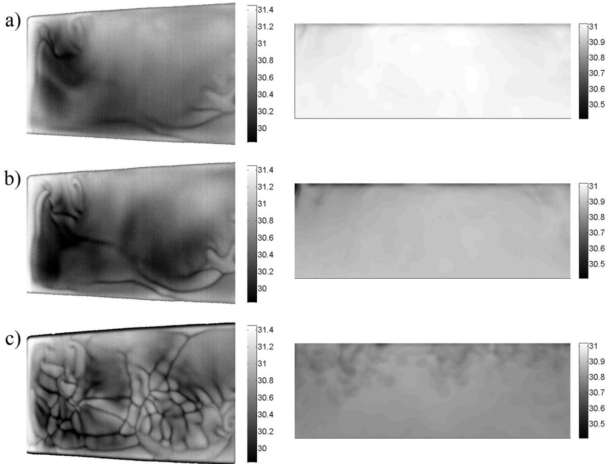
**Figure 10.** Water cooling from 31°C. Air temperature is 23.2°C, relative humidity is 25.5%. Water depth is 12 cm. Left column presents thermal imaging results for surface temperature (°C), right column shows simultaneous BOS measurements. Images in the upper row were taken 15 s after taking off the lid, middle row – 25 s, lower row – 45 s. [Click here](#) to toggle between color and grayscale images.
