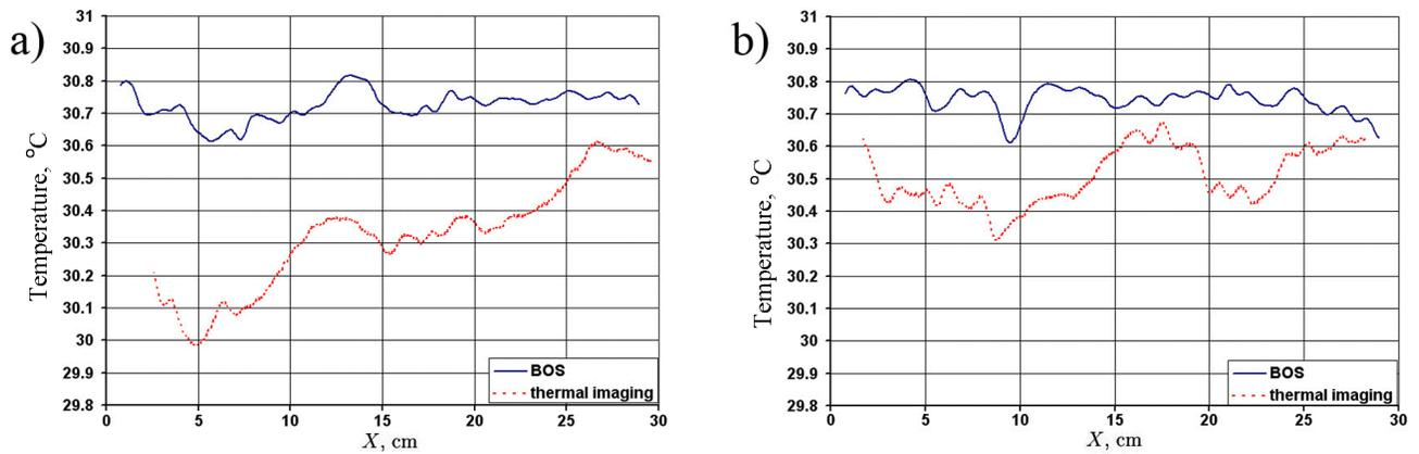
**Figure 11.** Comparison of temperature profiles along water surface measured by BOS and thermal imaging in the large tank a) 25 s, b) 45 s after taking off the lid. Thermal imaging distribution was averaged over the tank width.
