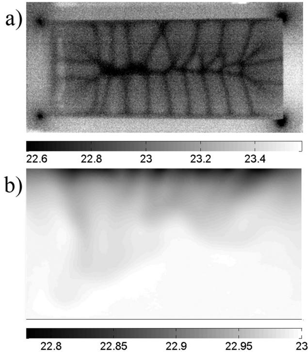
**Figure 8.** Temperature fields ( $^{\circ}\text{C}$ ) for evaporating ethanol. a) Surface temperature field observed by thermal imaging, b) side view of temperature distribution obtained by BOS. Images are taken 19 s after taking off the lid. [Click here to toggle between color and grayscale images.](#)
