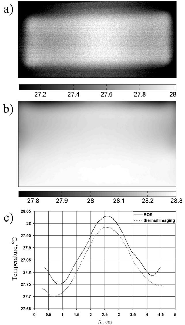
**Figure 7.** a) Water surface temperature field ( $^{\circ}\text{C}$ ) observed by thermal imaging device, b) side view of temperature distribution ( $^{\circ}\text{C}$ ) obtained by BOS, c) comparison of temperature profiles along water surface measured by BOS and thermal imaging. [Click here](#) to toggle between color and grayscale images.
