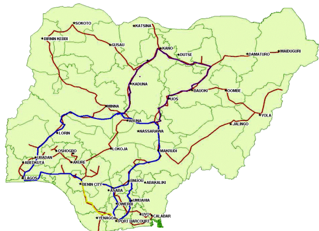
Figure 3. MTN Nigeria’s national microwave and fibre optic transmission network. Source: [Chukwuma et al., 2009], courtesy of MTN Nigeria.
