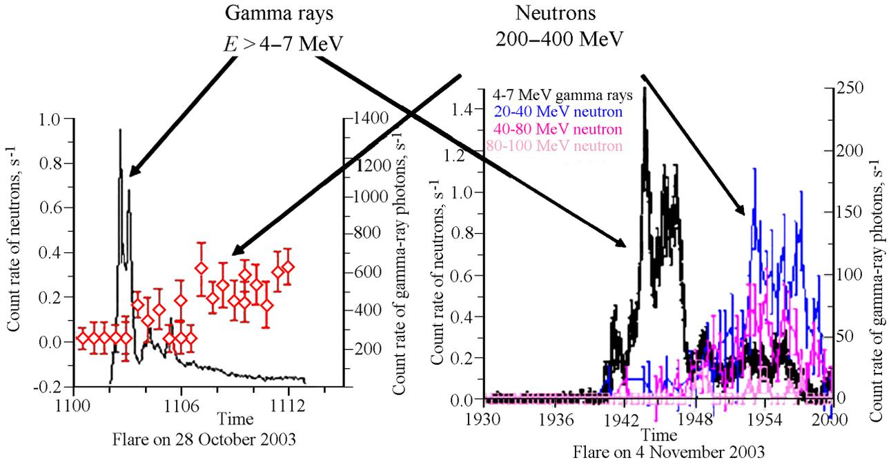
**Figure 9.** Fluxes of the gamma radiation of neutrons from the solar flares on 28 October 2003 and 4 November 2003. The spectrometer SONG of solar neutrons and gamma radiation.
