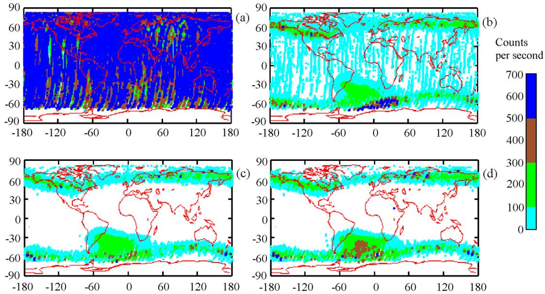
**Figure 17.** Maps of the emission of the nighttime atmosphere of the Earth drawn for four energetic intervals: a – 3–5 keV, b – 5–8keV, c – 8–16keV and d – 16–31 keV according to the data of the RPS-1 device obtained during a year of observations from 23 September 2002 to 23 March 2003 (winter).
