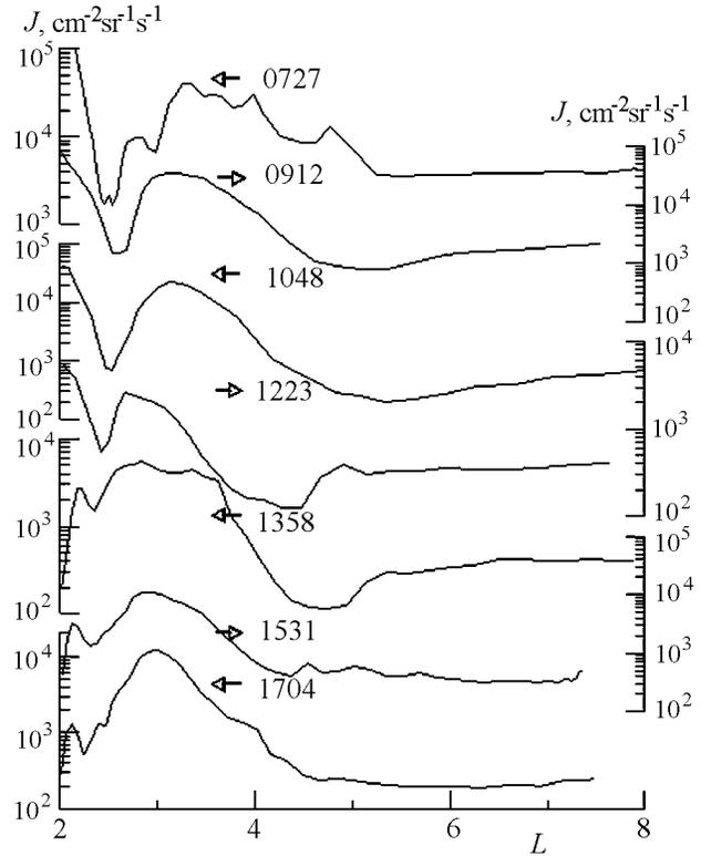
**Figure 14.** Changes in the structure of the radiation belt of electrons with  $E_e=0.3-0.6$  MeV at the development of the main phase of the 24 November 2001 magnetic storm (according to the CRM device data). The electron flux intensity is shown at the ordinate.
