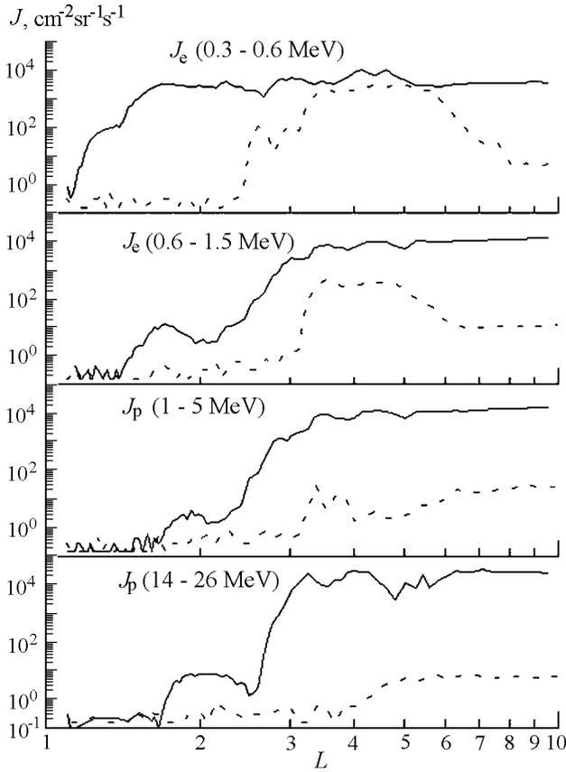
**Figure 11.** Changes in the distributions of electron ( $J_e$ ) and proton ( $J_p$ ) fluxes over  $L$ -shells illustrating the deformation of the magnetosphere and radiation belts and penetration of energetic particles into the magnetosphere and radiation belts in the period of strong magnetic storms on 28 October 2003 (dashed curve) and 29 October 2003 (solid curve). The SCR experiment.
