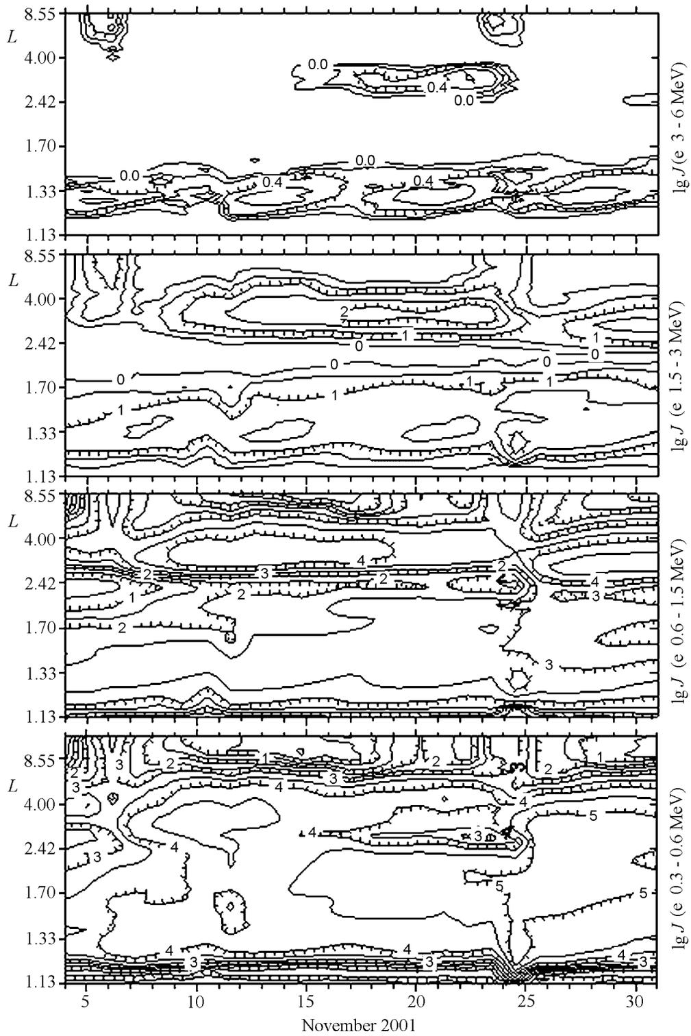
**Figure 15.** Changes in the structure of the electron radiation belt during the period 4–30 November 2001. Some isolines are marked by short perpendicular dashes. The dashes are directed to the intensity decrease. According to the data of the CRM device.
