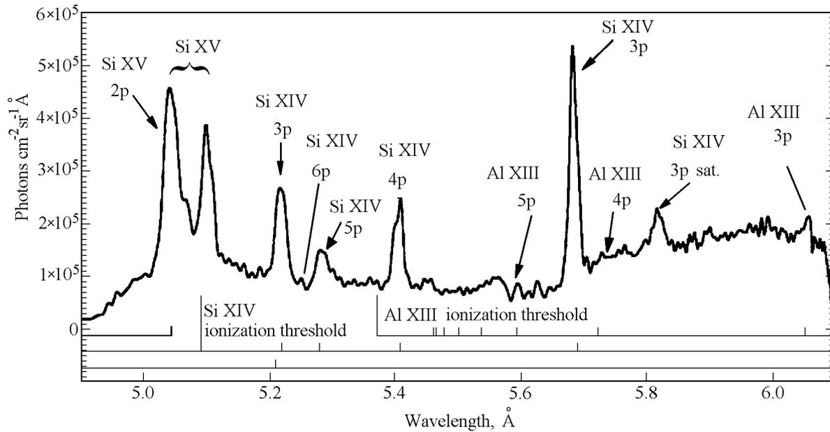
**Figure 7.** Spectral triplet of Si XV ion and lines of the helium-like ions Si XIV and Al XIII corresponding to the atomic transitions with high values of the  $n$  quantum number: from  $n = 3$  to the ionization threshold. The X-ray spectrometer RESIK.
