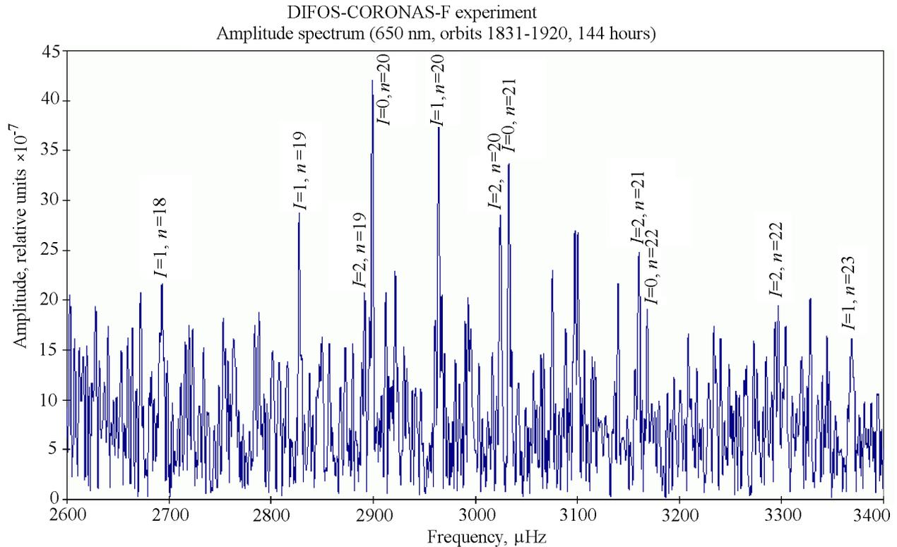
**Figure 1.** The power spectrum of the global oscillations of the Sun. The DIFOS experiment.
