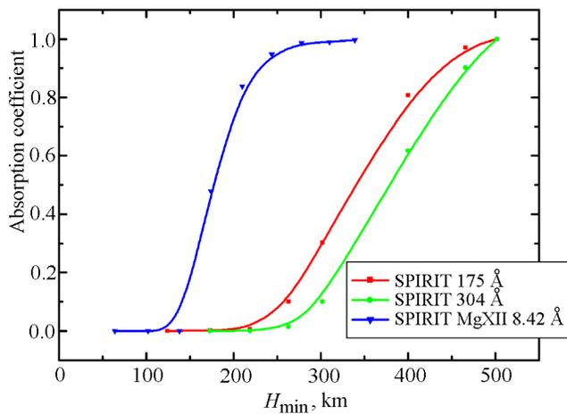
**Figure 18.** The dependence of the coefficient of the X-ray radiation absorption by the Earth’s atmosphere on the  $H_{min}$  height (the shortest distance between the Earth’s surface and the line connecting the Sun and CORONAS-F spacecraft). The SPIRIT experiment.
