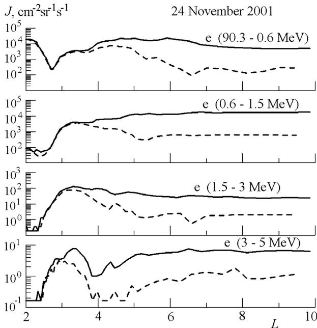
**Figure 13.** Increase in the electron fluxes during the first phase of the magnetic storm on 24 November 2001. The data obtained at the previous passage of the satellite (before the commencement of the magnetic storm) are shown by dashed curves.  $L$  is the magnetic coordinate (the number of the  $L$ -shell). According to the data of the CRM device.
