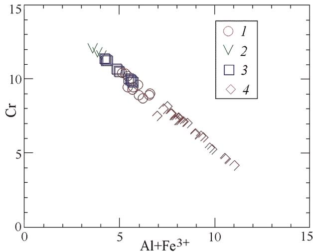
**Figure 16.** Cr/Al+Fe<sup>3+</sup> diagram for chrome spinels (calculated for 3 oxygen atoms) from the rocks of the layered series in the Aganozero Body: 1 – accessory chrome spinels from the rocks of the ultrabasic zone, 2 – chrome spinels from the ore-bearing layer in the Yakozero Body, 3 – from the main chromite unit, 4 – from a peridotite marker in the rocks of the gabbronorite zone.
