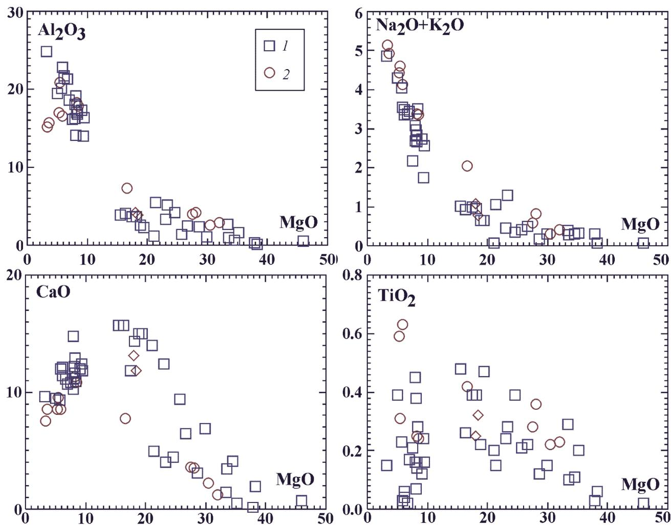
**Figure 17.** Percentages of oxides as a function of MgO in the rocks of the Burakovka Pluton. 1 – Aganzero Body, 2 – Shalozero–Burakovka Body.
