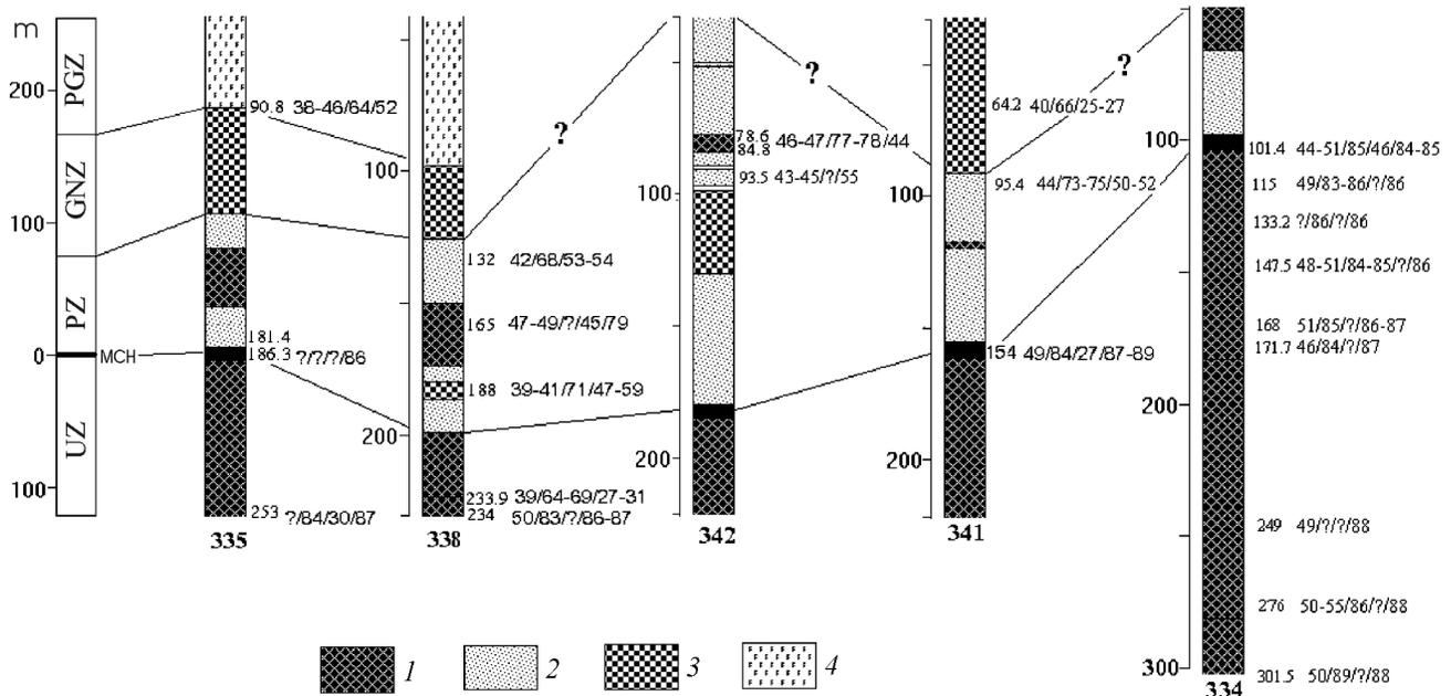
**Figure 9.** Structure of the pyroxenite zone from the holes drilled in the Shalozero-Burakovka Body. Shown in the figure are the numbers of core samples and the compositions of the main mineral phases: Cpx(En)/Opx(En)/Pl(An)/Ol(Fo). See Figure 3 for the legend.
