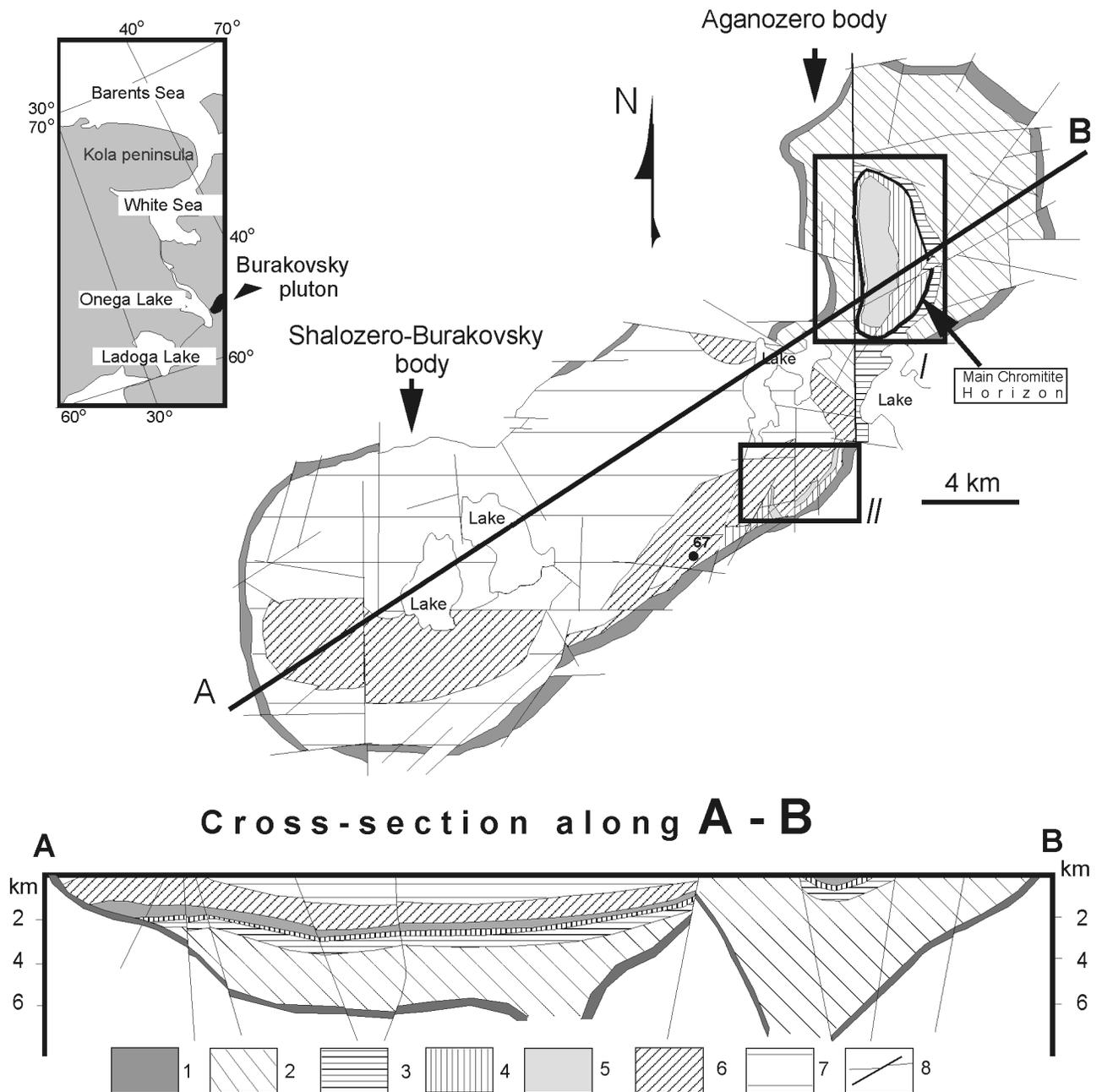
**Figure 1.** Schematic geological map of the Burakovka Pluton showing a marginal zone (1) and layered zones: 2 and 3 – dunite and peridotite zones of the ultrabasic zone, 4 – pyroxenite zone, 5 – gabbronorite zone, 6 – pigeonite gabbronorite zone, 7 – magnetite gabbronorite zone; 8 – faults; 9 – hole sites. The inset maps I, II, and III show the locations of the hole sites and profiles of study.
