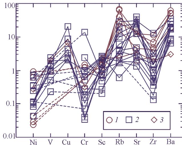
**Figure 20.** Distribution of trace and rare earth elements in the rocks of the Shalozero (1) and Aganozero (2) bodies and in the rocks of the marginal series in the Shalozero–Burakovka Body (3) normalized to the primitive mantle after Hoffmann [1988].
