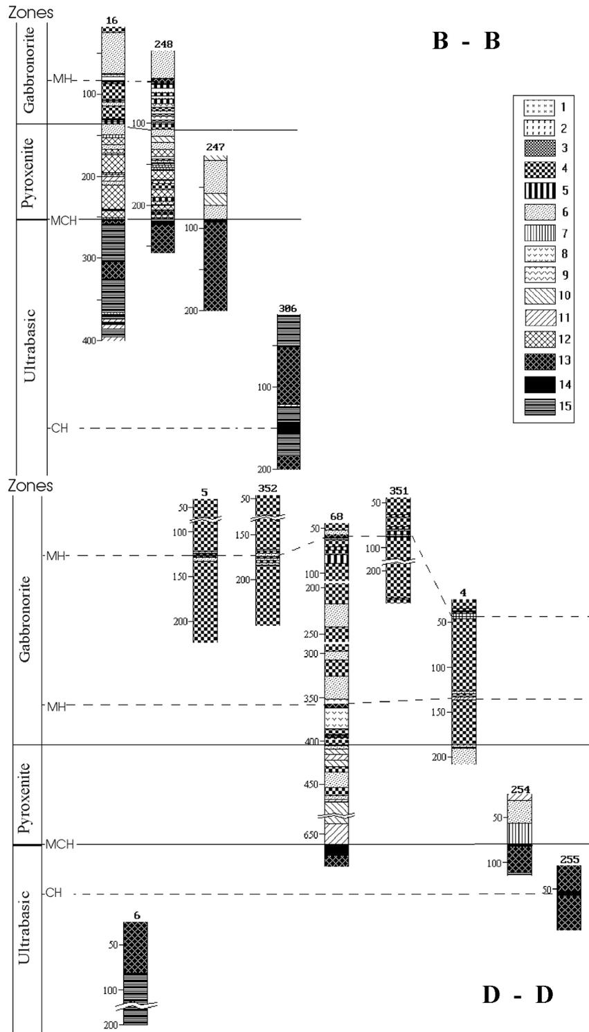
**Figure 3.** Schematic correlation of the holes along profiles B and D of the Aganzero body: 1 – quartz-feldspar rocks, 2 – pigeonite gabbronorite, 3 – magnetite gabbronorite, 4 – gabbronorite, 5 – gabbronorite-anorthosite, 6 – websterite, 7 – olivine websterite, 8 – orthopyroxenite, 9 – olivine orthopyroxenite, 10 – clinopyroxenite, 11 – olivine clinopyroxenite, 12 – wehrlite, lherzolite, and harzburgite; 13 – poikilitic peridotite, 14 – chromitite, 15 – dunite.
