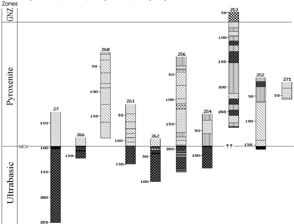
**Figure 7.** Structure of the pyroxenite zone of the Aganozero Body based on drilling data. See Figure 3 for the legend.
