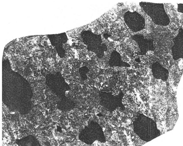
**Figure 8.** Relic sites of peridotite (dark) in a pigeonite augite aggregate from the base of the pyroxenite zone in the Aganozero Body.
