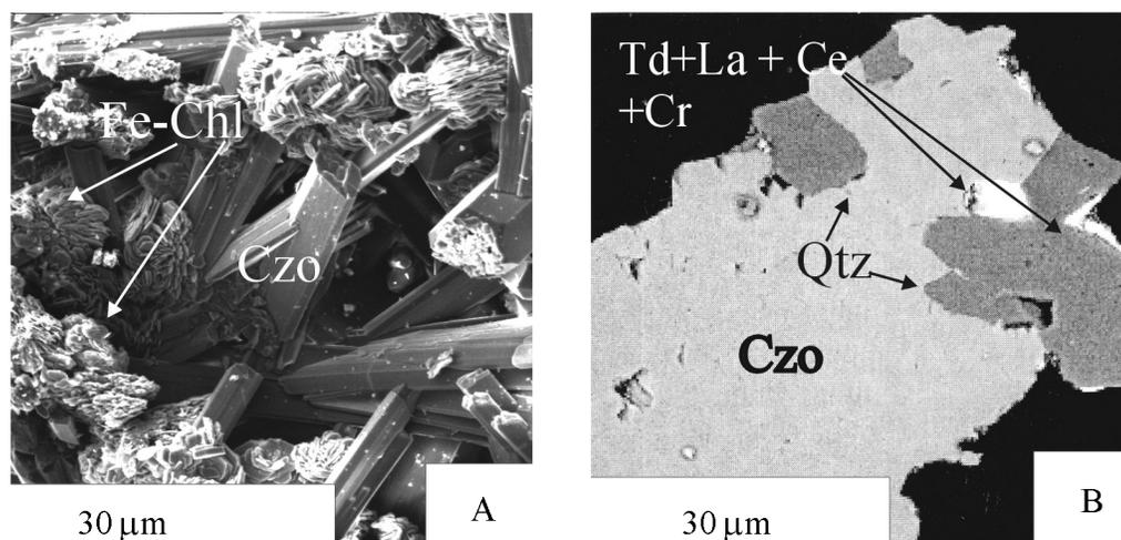
**Figure 7.** SEM photographs of the natural surfaces (A) and polished sections (B) of the aggregates of preore hydrothermal minerals from the outer zone of the Dukat orefield. One can see the close growths of the large grains of clinozoisite (Czo), quartz (Qtz), and Fe-chlorite (Fe-Chl) with the inclusions of C–Pb–Tl todorokite, rare-earth minerals, and eskolaite (Td + La + Ce + Cr).
