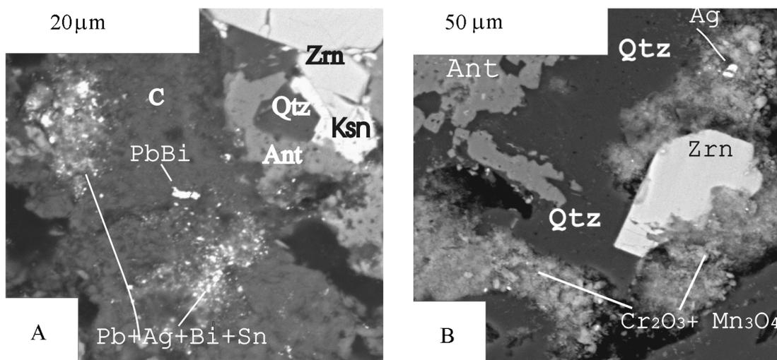
**Figure 5.** SEM photographs of the surfaces of polished sections showing idiomorphic grains of anatase (Ant), zircon (Zrn), quartz (Qtz), and xenotime (Xen). The microaggregate formed during the early mineralization phase (A) is enriched in carbonaceous matter and graphite (C) and in native Ag, Pb, Sn, and Bi. The microaggregate formed in oxidation environment (B) is enriched in Mn hydroxides, eskolaite  $\text{Cr}_2\text{O}_3$ , and native Ag.
