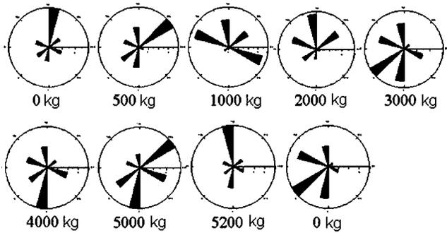
**Figure 11.** The azimuthal distribution of the supersonic wave velocity (data of the 3-D transducers). The moment of arrival of the wave according to the moment the signal began to appear. Symmetric routes.
