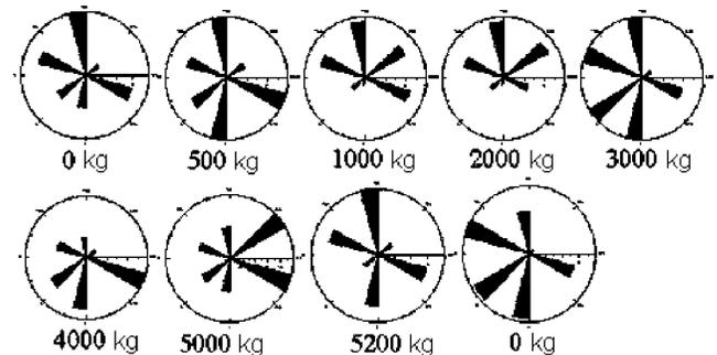
**Figure 10.** The azimuthal distribution of the supersonic wave velocity (data of the 3-D transducers). The moment of the wave arrival determined from the first half-cycle of the wave crossing the maximum. Symmetric routes.
