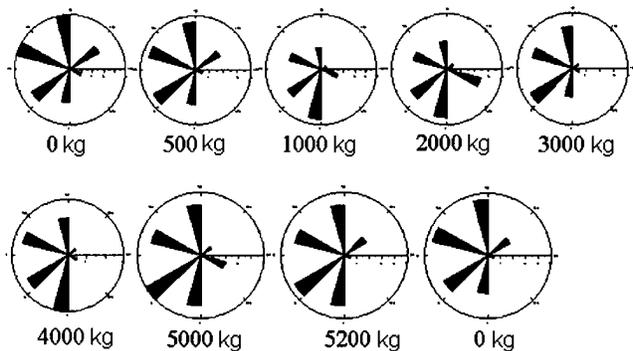
**Figure 12.** The azimuthal distribution of the supersonic wave velocity (data of the 3-D transducers). The sounding routes are arranged at an angle of 45°.
