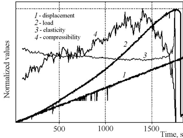
**Figure 4.** Loading curve (black) at a constant rate of deformation (blue). The corresponding elasticity factor (black broken line) and the volume dynamic compressibility index. Max. displacement = 1.52 mm, max. load = 4.52 t.
