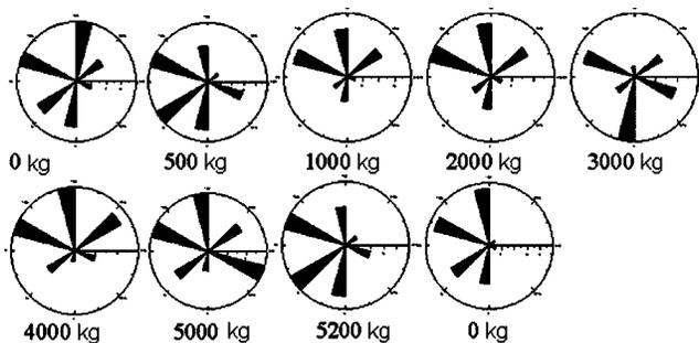
**Figure 9.** The azimuthal distribution of the supersonic wave velocity (accelerometer data). The moment of the wave arrival determined from the first half-cycle of the wave crossing the maximum. Symmetric routes.
