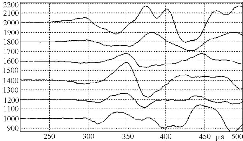
**Figure 8.** The nature of the wave pattern along coordinate *Y* on the sample before loading.
