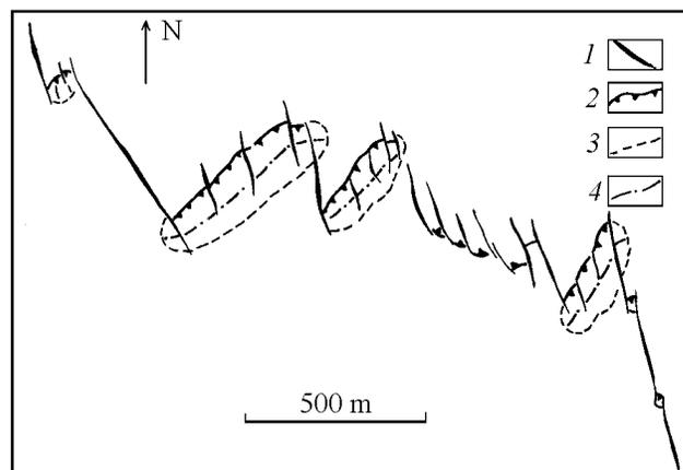
**Figure 7.** The structure of a seismic fault in the area of the watershed between the Taldura and Kuskunnur rivers. (1) seismic trench or open fracture; (2) dextral pressure ridges thrust scarp; (3) pressure ridge outline; (4) dextral pressure ridges axis.
