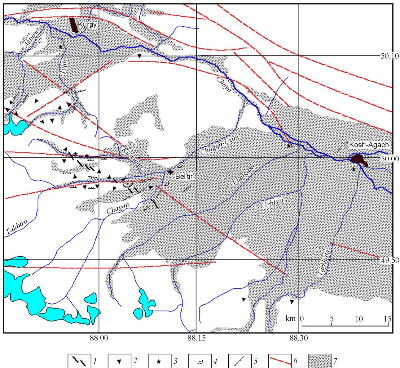
**Figure 1.** Map of seismic ruptures: (1) seismotectonic faults; (2) rockfalls; (3) ground dilution; (4) landslides; (5) seismogravitational breaks and downward movement of the slopes; (6) faults rejuvenated in Neogene-Quaternary time [Dvyatkin, 2000]; (7) Quaternary alluvial, lacustrine, and glacial deposits.
