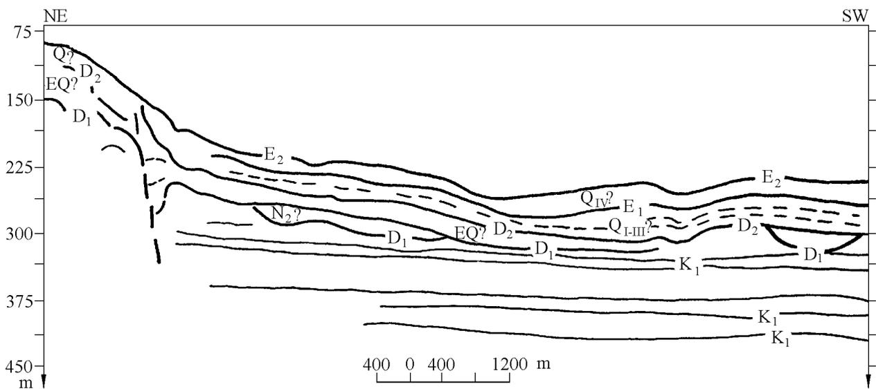
**Figure 20.** Interpretation of the record displayed in Figure 19 showing drape sheets of Quaternary seismic units.
