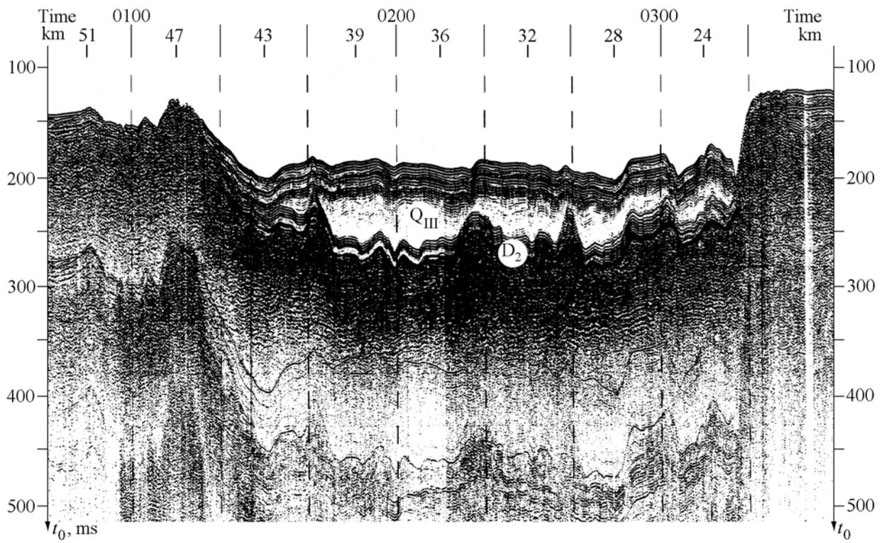
**Figure 21.** Example of seismic record of Cretaceous and Quaternary seismic units.
