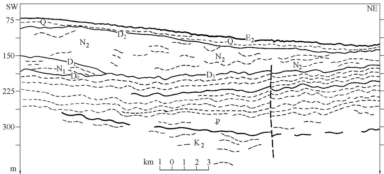
**Figure 14.** Interpretation of the seismic record displayed in Figure 13 showing the geometries of the tops and bottoms of the Paleogene, Miocene, Pliocene, and Quaternary sequences.
