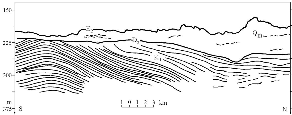
**Figure 8.** Interpretation of the record displayed in Figure 7 showing pre-Quaternary erosional truncation.
