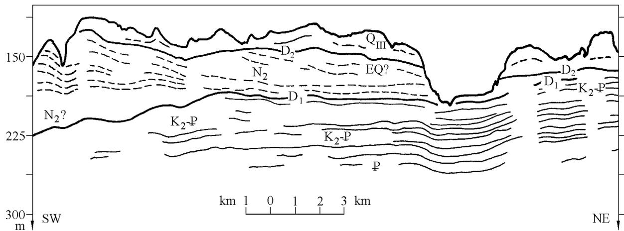
**Figure 12.** Interpretation of the record displayed in Figure 11 showing pre-Pliocene and recent erosional truncations.
