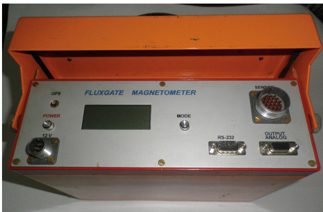
Figure 6. Magnetic variational station LEMI-008.
