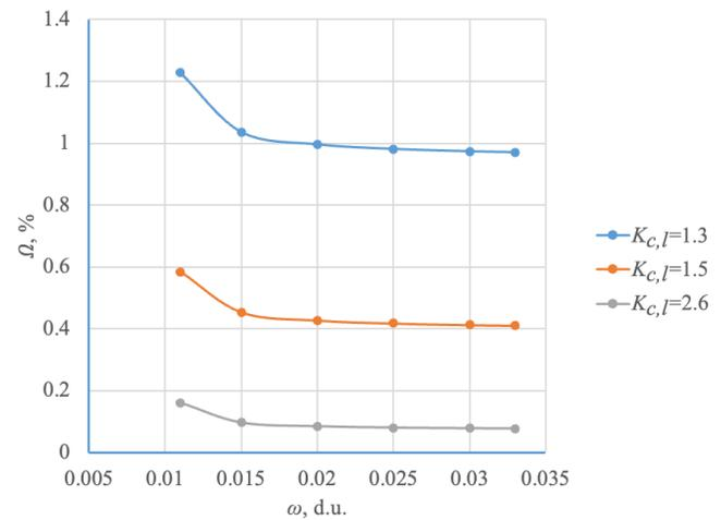
**Figure 5.** The family of dependences for current values of outburst danger criteria  $K_{c,l}$  on the methane concentration in the vicinity of the face working and the value  $\omega$ , opposite to the coal strength.
