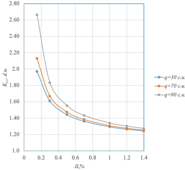
**Figure 4.** The dependence of the limit current outburst danger indicator  $K_{c,l}$  on the methane concentration  $\Omega$  (%) for different coal strength values  $q$  (c.u.).
