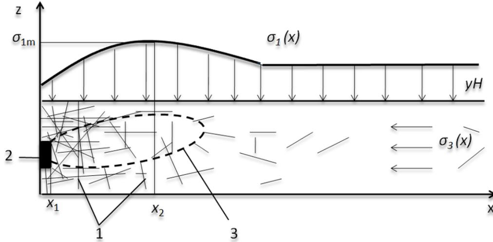
**Figure 3.** Squeezing the coal block out of the outburst cavity mouth.
