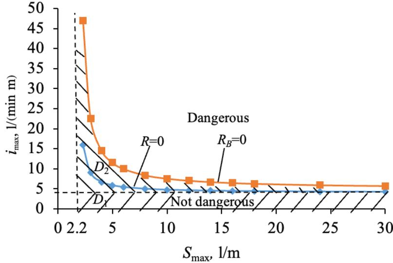
**Figure 1.** The dependence of the outburst danger indicator  $R = 0$  on the initial gas-emission rate  $i_{\max}$  and the drilling fines output  $S_{\max}$  when  $a = 4$  and  $b = 6$ .
