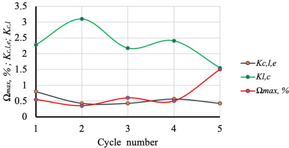
**Figure 6.** The dependence of the critical values of  $K_{c,l,e}$  and  $K_{l,c}$ , indicators and methane concentration in the atmosphere of the working  $\Omega_{max}$  on the number of the face working driving cycle.
